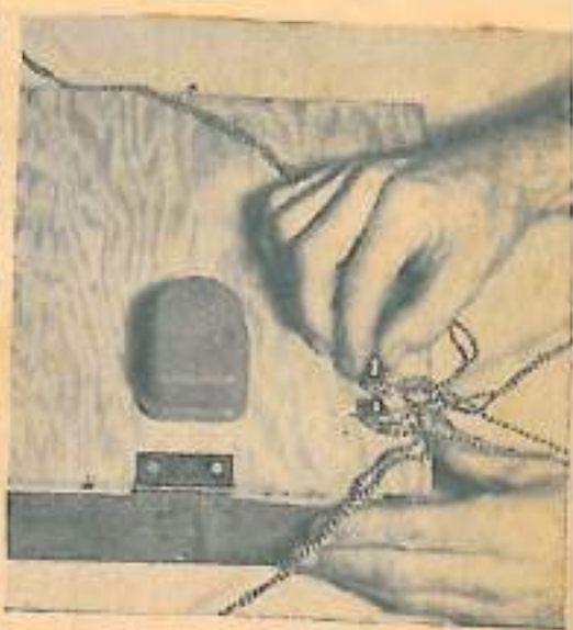
battery clip to one post of buzzer; second buzzer post to second terminal. Attach key wires to terminals.
